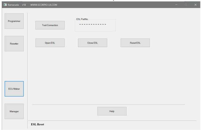
4. Press **Test Connection** to verify wiring then proceed with **Reset ESL**
